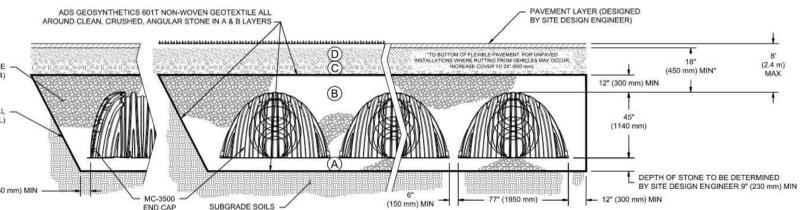
ADS GEOSYNTHETICS 601T NON-WOVEN GEOTEXTILE ALL AROUND CLEAN, CRUSHED, ANGULAR STONE IN A & B LAYERS
